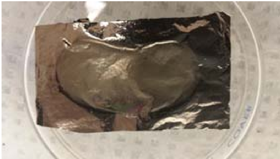
FIG. 2. Arc-shaped 438 \mu\text{g}/\text{cm}^2 ^{nat}\text{Gd}_2\text{O}_3 target on 2 \mu\text{m} Ti backing.
